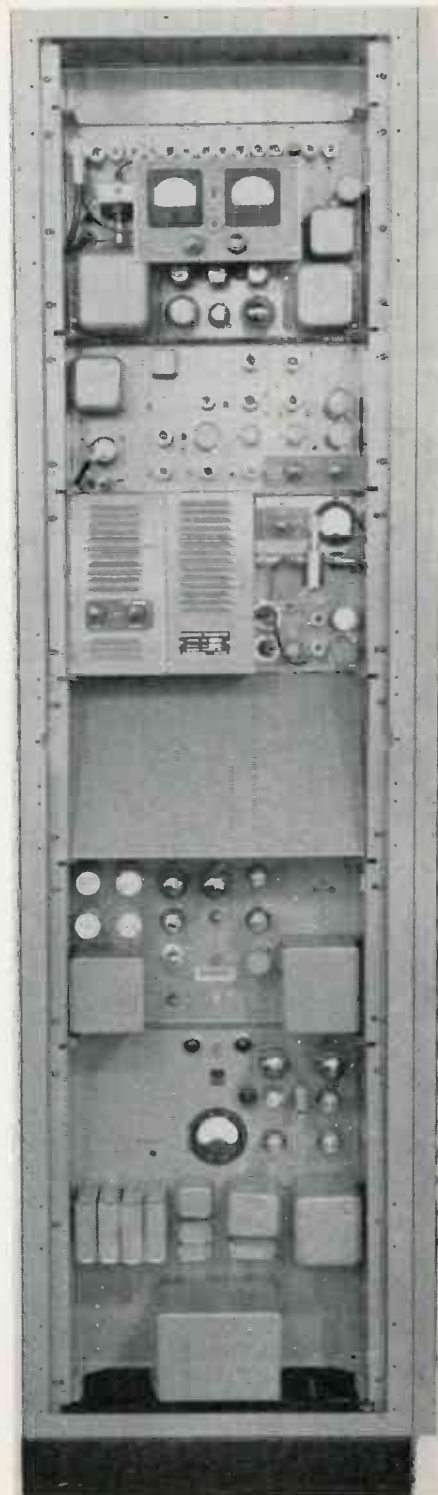
Fig. 2 — Sarkes Tarzian M/W Equipment, Model MWF-1C, long-range microwave relay.
